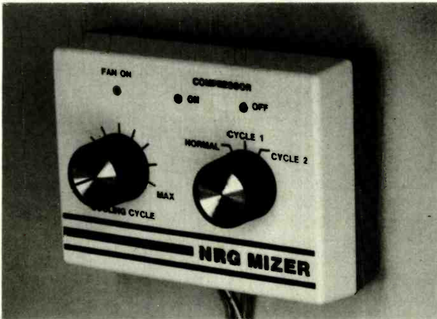
FIG. 5—USING A PLASTIC case for the project allows you to simply use double stick foam tape to mount it to the wall.
