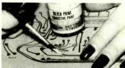
FIG. 10—SILVER PAINT, though expensive, is excellent for repairing hairline cracks in traces.
