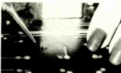
FIG. 7—MAKING A JURY-RIGGED strain relief using solder.
