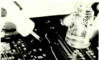
FIG. 8—USE NAIL POLISH to secure the wire to the board. It works better than any glue we've tried.
