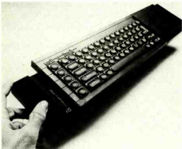
FIG. 2—THE NEW SINCLAIR QL shown with a prototype of the forthcoming QL 0.5megabyte RAM pack, connected via the QL's internal expansion slot.
