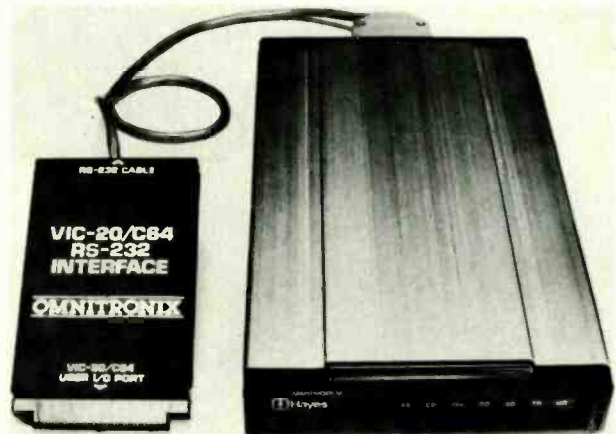
THE VIC20/C64 RS-232 interface from Omnitronix plugs into a TTL user port and provides true RS-232 I/O.
