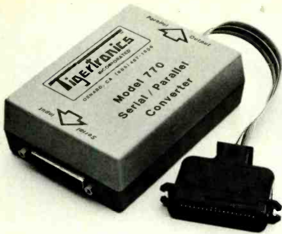
TIGERTRONICS MODEL 770 plugs into the Color Computer's serial input/output and converts serial data to a Centronics-type output.
