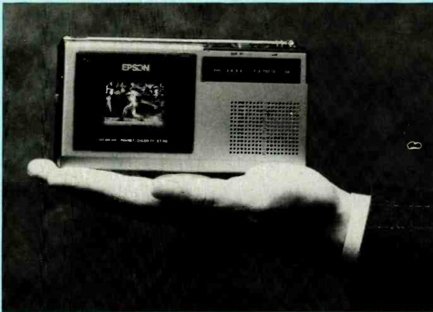
FIG. 4—THE EPSON ELF is as small as a paperback book, weighs just over one pound, and can operate indoors or out. It makes use of Epson's flat-screen color liquid-crystal display.
