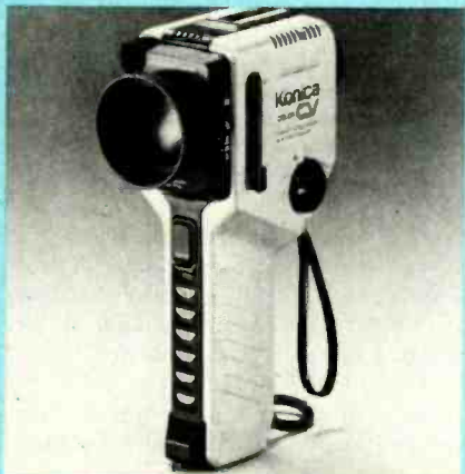
FIG. 3—KONICA'S CV-301 sports a stubby profile despite using a tube pickup. That is possible because of the location of the pickup—it is mounted vertically in the handle.
