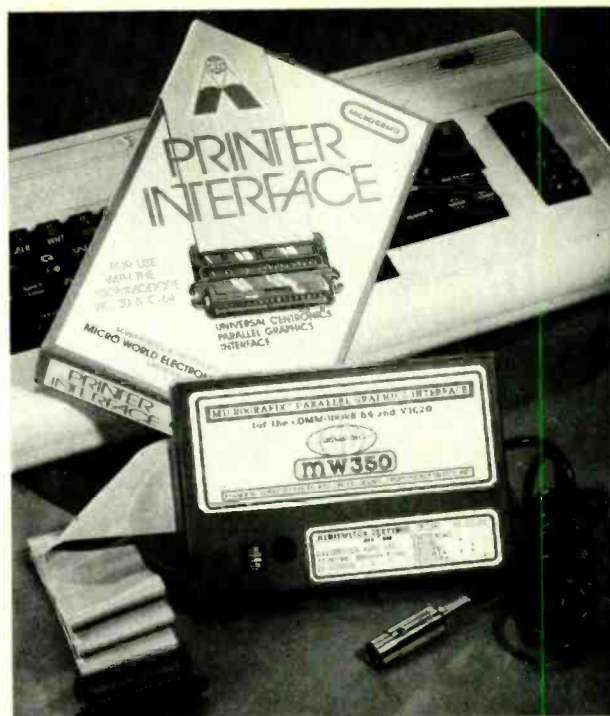
THE CONNECTION, FROM MICROWORLD, connects the RS-232 serial output of the Commodore 64 or the VIC-20 to standard Centronics parallel so you can print standard ASCII on any Centronics-input printer.
