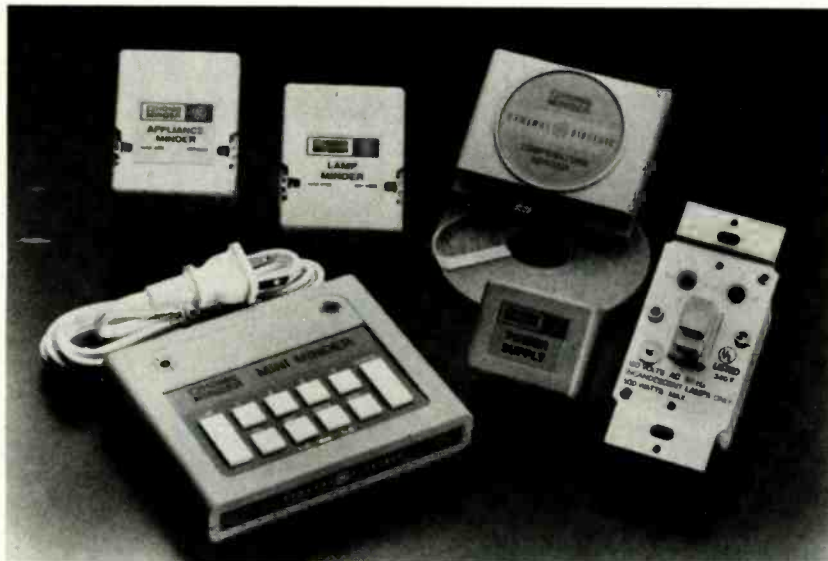
MODULES THAT MAKE THE HOMEMINDER WORK. The ApplianceMinder (left top) and LampMinder (next right) connect any lamp or appliance to the system. The Light Switch module (right) installs like a dimmer switch and connects indoor or outdoor lights to the HomeMinder . The Temperature Minder module (second from right) is attached under the existing thermostat and regulates heating and air conditioning. It connects to the power supply module beneath it. The MiniMinder remote control (lower left) can operate up to eight lights and appliances from any electric outlet in the home.
