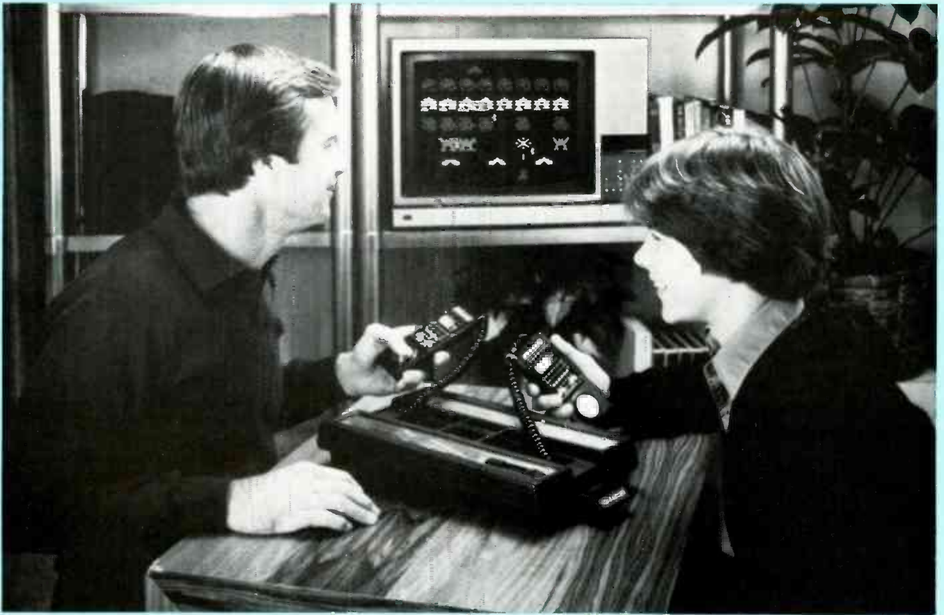
ALL-IN-ONE HAND CONTROLLERS are featured in the Intellivision videogame unit. Those hard-wired controllers slip into pockets on the console when not in use.
