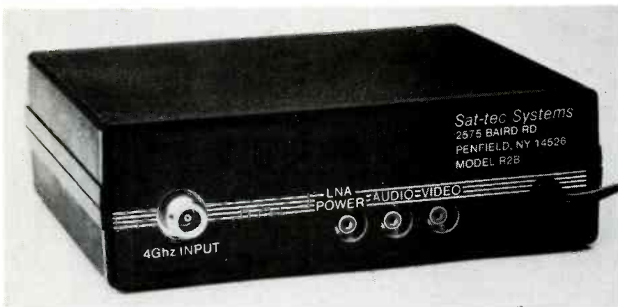
FIG. 26—REAR-APRON CONNECTIONS for the satellite TV receiver. If you are not building the kit, any layout that is convenient may be used.
