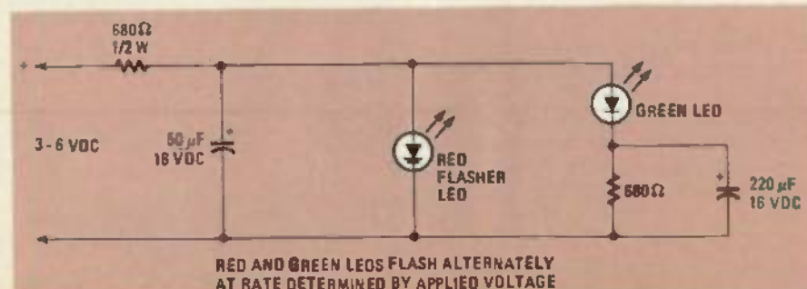
FIG. 7—RED AND GREEN LED's flash alternately at a rate determined by the applied voltage.
