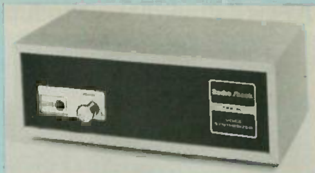
VOICE SYNTHESIZER adds speech capability to the computer.
