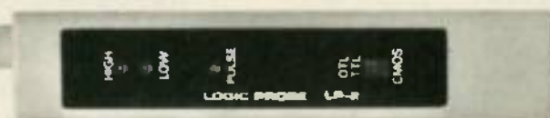
Logic Probe LP-2. All the basic features of LP-1, with pulses as fast as 300 nanoseconds, to 1.5MHz. Doesn't have LP-1's memory feature, but features even lower price: $28.00*.
