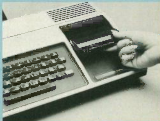
PLUG-IN COMMAND MODULES contain programs in ROM.
