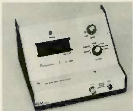
FIG. 7—THIS LAYOUT works well, but is not ideal. Output jacks and "level" pot should be located closer to one another to keep leads short.
