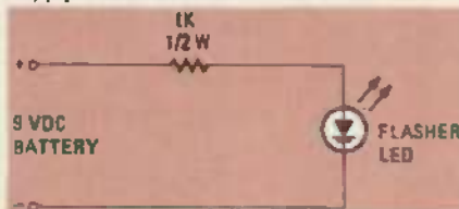
FIG. 2—POWER can be obtained from a 9-volt source if a dropping resistor is used.
