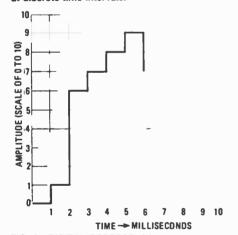
FIG. 3—DIGITAL REPRESENTATION of analog waveform shows rough approximation due to low resolution analog-to-digital conversion.
