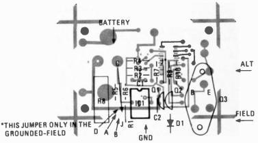
FIG. 5—PARTS PLACEMENT GUIDE for the voltage regulator. Note that the jumper between R7 and R9 is used only when the circuit is used with a grounded-field alternator. A jumper must be installed between point "A" and point "B", "C", or "D", depending on the desired temperature coefficient.
