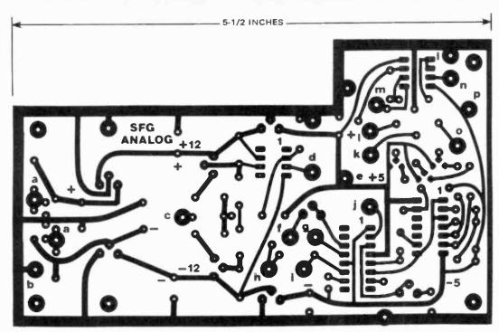
FIG. 3-FOIL PATTERN for the analog circuit board.
