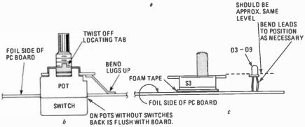
FIG. 8—HOW POTS, SWITCH, AND LED's are mounted on the PC board. Diagram at a shows how potentiometer lugs are soldered to pads on the PC board. Sketch at b shows how to shape the control lugs before soldering and c shows details of switch S3 and LED mountings.
