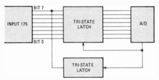
FIG. 3—ASYNCHRONO:JS OPERATION of A/D converter can reduce the number of required I/O ports to one in an I/O-based interface.
