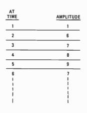
FIG. 2—DIGITAL CONVERSION of analog signal requires sampling the amplitude of the analog signal at discrete time intervals.
