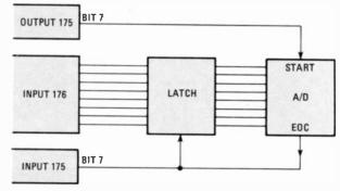
FIG. 2—I/O BASED INTERFACE requires three I/O ports. One port handles the data while the other two control the A/D converter.
