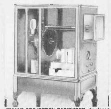
JENKINS PROJECTIOM RADIOVISOR, developed in 1931, used deficrest's new neon-crater tube and a 1-inch scanning disc with sixty ½-inch lenses to throw a flying-spot image on the rear of the ground-glass viewing screen.
