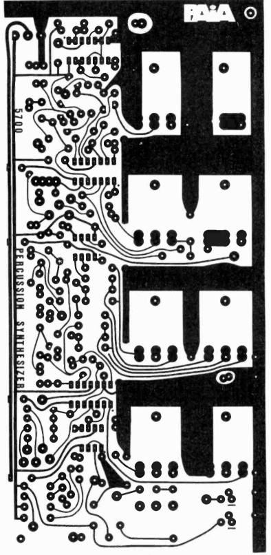
FIG. 5—PATTERN for one drum-synthesizer module. You need four modules to duplicate The Drum.
