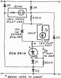
\* BREAK HERE TO INSERT TRANSFORMER WINDING, DI-DS SWITCHING DIODES; I AMP, GOO PIV, SILICON
