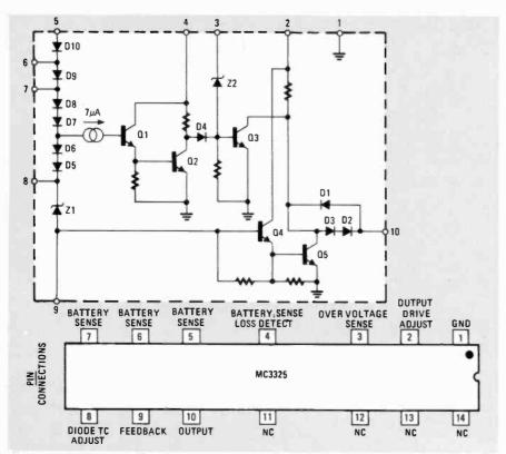
FIG. 2—CIRCUIT DIAGRAM and pin-out for the Motorola MC3352 voltage regulator IC.
