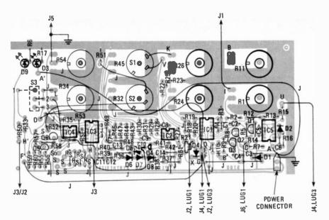
FIG. 6—HOW PARTS ARE POSITIONED on the synthesizer modules. The four R<sub>8</sub> resistors are installed only on the module for the fourth channel. The diagram also shows jumpers and conpections to off-board components.
