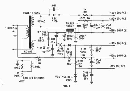
The +145-volt supply comes straight off the AC line, through diode D103. Stock filtering is used to smooth out the supply. From that the +135-volt and +20-volt lines are taken, reduced by resistors.
