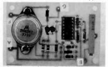
COMPLETED REGULATOR PC Board. Letters A, B, F and G show connecting points for alternator, field, battery and ground.
