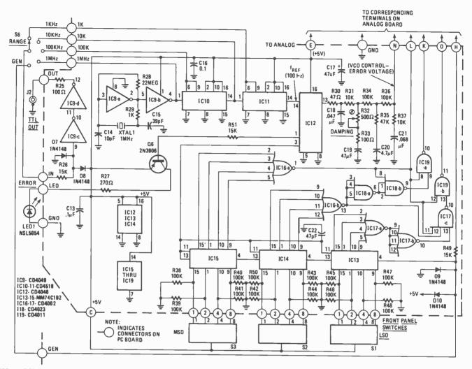
FIG. 1—SCHEMATIC DIAGRAM of the digital circuitry used in the SFG. The many output frequencies are all derived from the 1-MHz crytal and a series of programmable frequency dividers.
