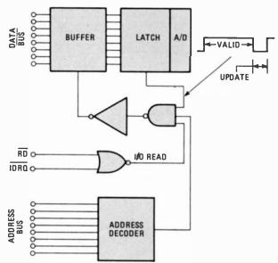
FIG. 6—DIRECT CONNECTION of A/D converter to microprocessor.
