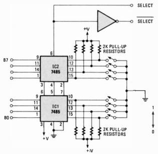
FIG. 5—ADDRESS DECODER using two 4-bit magnitude comparator iC's and a DIP switch permits easily changing the address of the I/O port.
