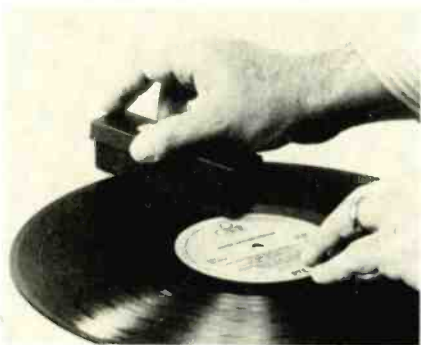
FIG. 4—BUFFING PAD is used to evenly spread Permostat solution over record surface.
