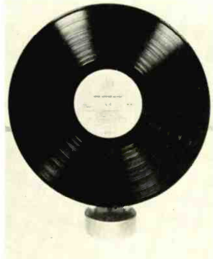
FIG. 6—PERMOSTAT-TREATED RECORD after being exposed in dust chamber.
