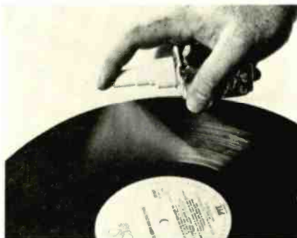
FIG. 3—PERMOSTAT LIQUID is applied directly to record surface via a hand pump.
