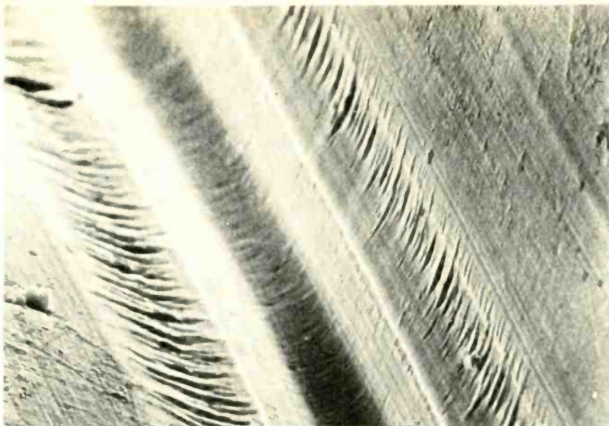
FIG. 7—SINGLE RECORD GROOVE of untreated record after 100 plays as viewed through electron microscope.
