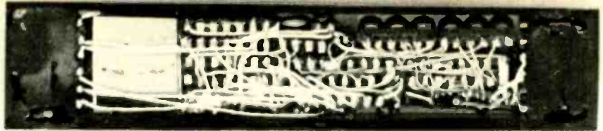
SMALL SIZE of probe-type frequency counter is due to IC "bricklaying" construction technique. IC's are glued together for maximum use of allotted space.
