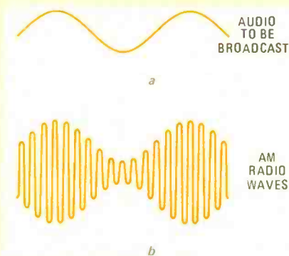
FIG. 1—AMPLITUDE MODULATION. The audio signal shown in a modulates the amplitude of the carrier wave as shown in b .
