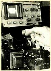
FIG. 5.—TO CORRECT FAULTY DUAL-SWEEP curve in Fig. 4-c, realign FM sound-detector coil at end of IF strip, while observing curve.
