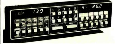
AUTOMOTIVE COMPUTER provides motorists with a driver controlled information center with 24 functions. At a touch of the button, vehicle location, trip information, time of day and fuel economy data can be displayed on the LED digital display. The unit is expected to retail for \$400.
