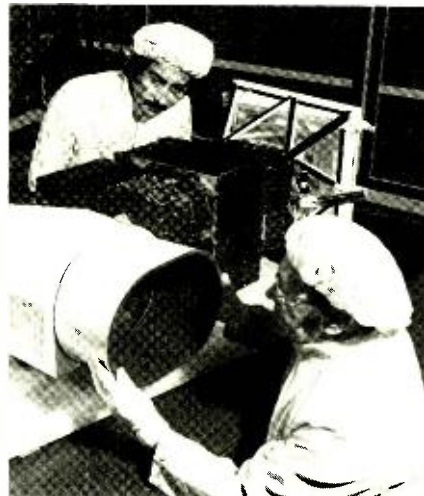
MULTISPECTRAL SCANNER (MSS) can take thermal photos of the earth at night. Here, Hughes Aircraft technician examines instrument's aperture, housing reflective mirror and telescope to record earth-surface images.
