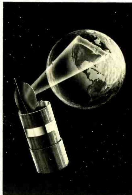
ANIK C SPACECRAFT, being built by Hughes Aircraft for Telesat Canada, will link southern Canada's cities from coast to coast (shown in artist's conceptual above). The satellite will provide telecommunications services in super-high-frequency range of 12 to 14 GHz.
