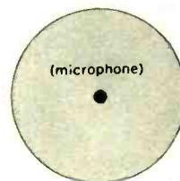
OMNIDIRECTIONAL MICROPHONE has a typical pick-up pattern as shown.
