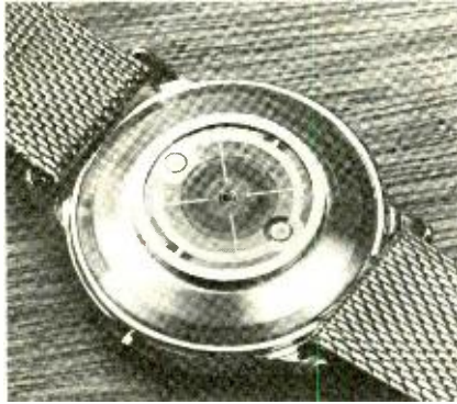
THE ORR HEARTBEAT TRANSDUCER consists of a light-emitting diode surrounded by a ring-shaped photovoltaic detector. The whole is designed to fit on the back panel of a standard wrist watch.
