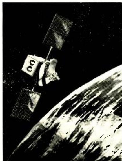
RCA SATCOM-1 SPACECRAFT, shown above as it would look if the photographer could get near enough to take a picture, is equipped with 24 transponders—double the communications capacity of any conventional satellite now in orbit. The solar panels have 71 square-feet of silicon cells always oriented toward the sun.
