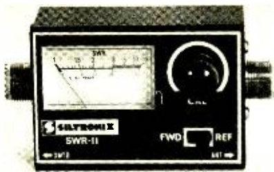
FIG. 8—STANDING-WAVE-RATIO bridge reads relative forward power or reflected power and SWR.
