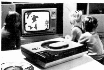
VIDEOPLAYER developed by Philips to play its VLP (Video Long Play) discs. Signal is fed to set's antenna terminals.
