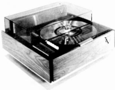
MCA DISCO-VISION PLAYER for single disc. Player uses laser read-out and feeds the antenna input of a standard TV receiver.
