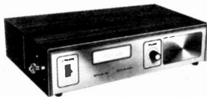
FIG. 4—THE DECODER used in the BTVision system. The built-in amplifier and speaker provide better sound than most TV sets.
