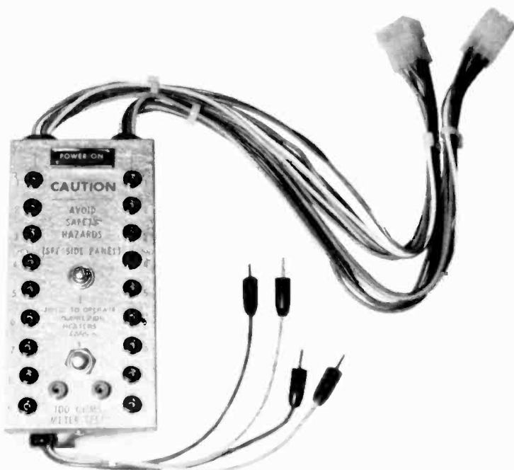
THE REFRIGERATOR ANALYZER checks the refrigerator's controls and components through connectors behind a bottom-front panel. Test leads are for ohmmeter resistance checks.
