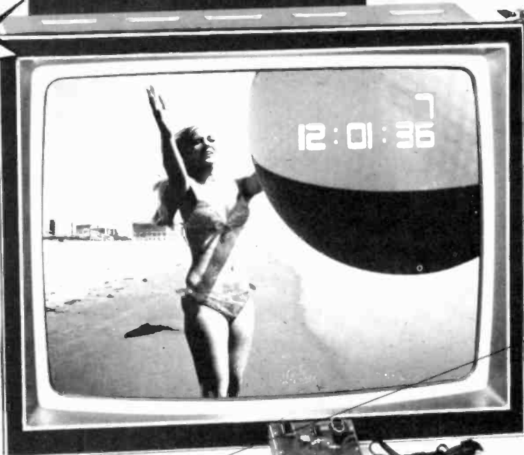
NTS DIGITAL GR-2000 SOLID STATE COLOR TV WITH 315 SQ. IN. PICTURE AND VARACTOR DIGITAL TUNING
