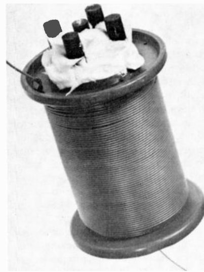
EXPERIMENTAL SUPER-LOOPSTICK is shown less shield. Rods are 5/8-inch long. Figure of merit is around 2. Resonating capacitor is around 235 pF.
