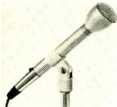
A popular microphone in the broadcast and entertainment field is the 635A by Electro-Voice. It has a built-in, four-stage blast filter for close-up work. It has an omnidirectional pickup pattern.
