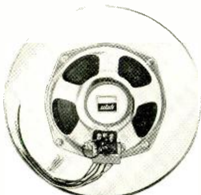
Many PA speakers, like Utah's above, have built-in transformers. At right is the Bogen MTX30B amplifier and the Utah SND-3 sound column.
