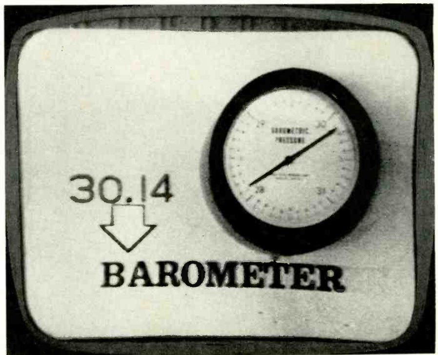
Fig. 1—Pincushioning is concave curvature in the raster edges. It is due to tube-screen geometry and is a fairly common trouble on large-screen TV sets.
