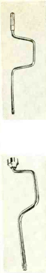
Fig. 14—Speeder is a crank to speed-up the work. Looks and operates very much like a carpenter's brace and bit. At the left is the Ovatomna H-283. At the right is Husky CB-85.
