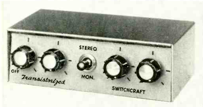
Fig. 2—Stereo mixer with solid-state amplifier eliminates loss problem, and can blend signals for left and right channels.
