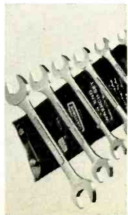
Fig. 1—The usual open-end wrench is double-ended, has parallel jaws, and each head is set at a 15-degree angle with respect to the plane of the handle. Craftsman model 4455, six-piece open end wrench set is shown
