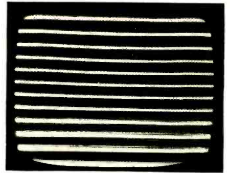
Fig. 5—Faulty thermistor in vertical output caused this linearity defect.
