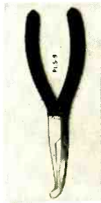
Fig. 12—Duckbill pliers have wide flat tips like the unit shown here. Normally there is no offset to the tips, but it is available in the Williams model PL-10.
