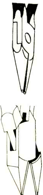
Fig. 6 — Lap joint (left) or box joint (right)? The lap joint is the most common type used and can develop wobbles and result in jaws getting out of alignment. Box joints are more costly, but do last longer.
