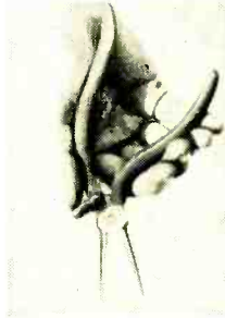
Fig. 8—Curved pliers handles can improve comfort and reduce fatigue when pliers are used for long periods. In the Klein model D-366-6C shown you can also note the coil spring that keeps its jaws open. The thumb rest is an extra not always found in tools.
