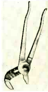
Fig. 13—Tongue-and-groove pliers are really extensions of the slip-joint plier principle. The important point is that the jaws stay parallel even when large diameter nuts have to be held firmly. The unit shown is made by Owatonna Inc.
