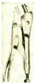
Fig. 17—Lever wrench pliers are great if you want to loosen a nut that has rounded corners as well as items that are normally round. P&C model 1219-R.
