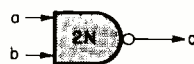
B- BASIC 2-INPUT NAND LOGIC SYMBOL (POWER CONNECTIONS USUALLY OMITTED FOR SIMPLICITY)
