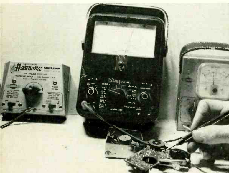
Instruments for transistor-radio fixing: A broadband signal generator, a volt-ohm-milliammeter and a battery eliminator.
