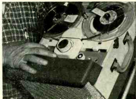
Tilting the machine to different positions is one way to check for unusual noises.
