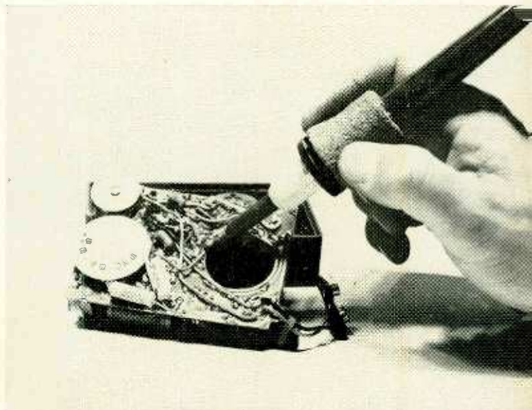
Another case of a drop breaking the circuit board; opens were bridged with insulated wire to correct the trouble.
