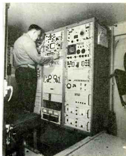
Calibration and service instruments are used to check out telemetry devices.
