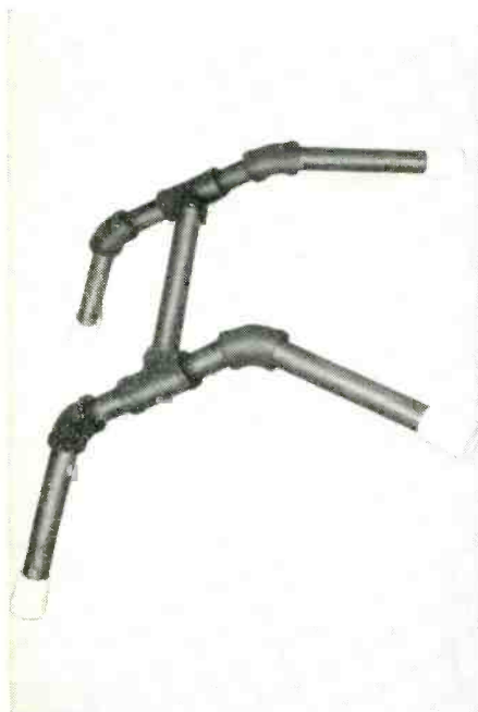
The assembled pipe sections form the saddle mount. Note white rubber feet.
