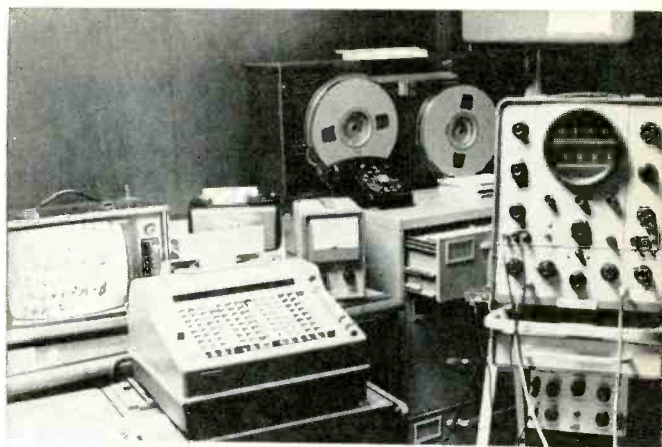
DUD monitor (left) displays repair instructions. Computer programmer is in foreground, tape memory and tech files behind.
