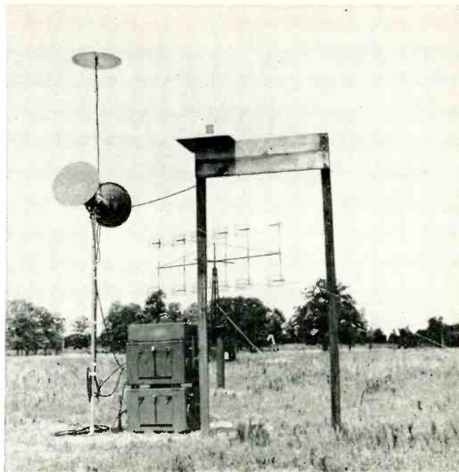
Antennas and equipment cases contain radar-range transponder, central timing recorder and aircraft tracking units.
