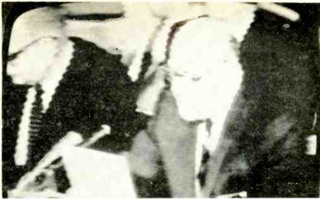
Horizontal afc hunting, caused by afc filter overcorrection.
