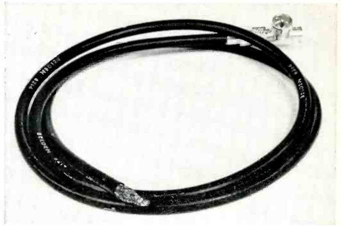
Stub has a tee connector at one end, a short at the other.
