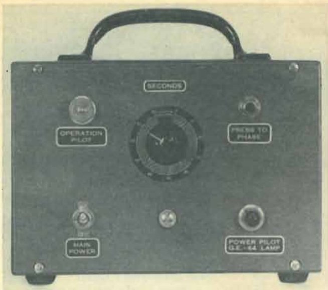
Neat labeling enhances front panel of the vacuum-tube timer. It's also a good idea to tag back-panel controls and switches.
