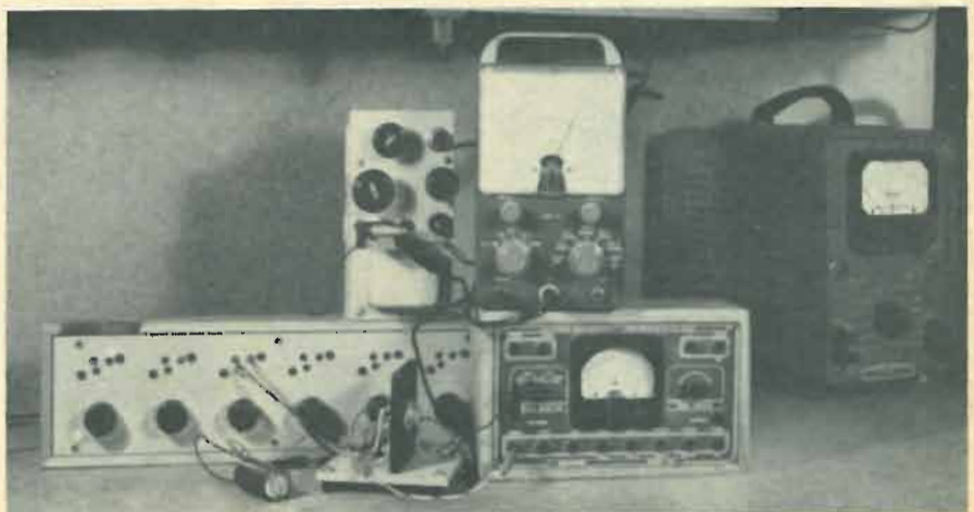
Power transistor provides load for making measurements on this regulated supply.
