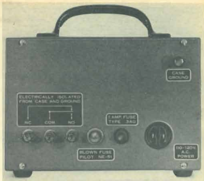
Neat labeling enhances front panel of the vacuum-tube timer. It's also a good idea to tag back-panel controls and switches.
