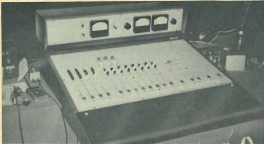
The console was designed for maximum operator convenience, to reduce possibility of error. Slide-type vertical attenuators conserve space on panel and are easy to use.
