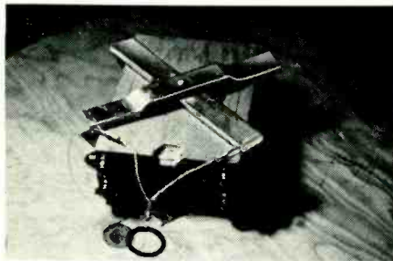
Underside of turntable assembly. Levers mount on plywood sandwich and turntable.
