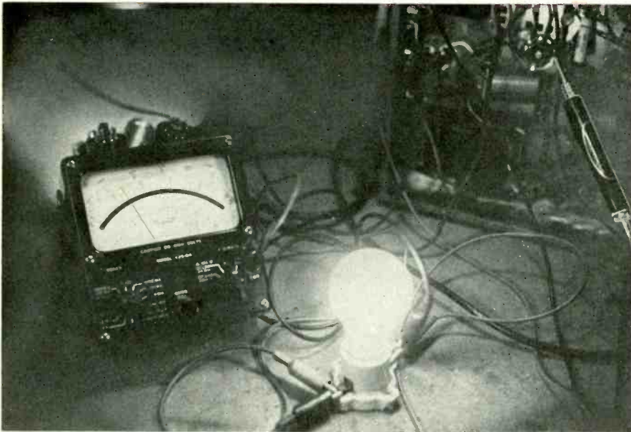
House lamp makes an acceptable dummy load for high-power amplifiers in an emergency.
