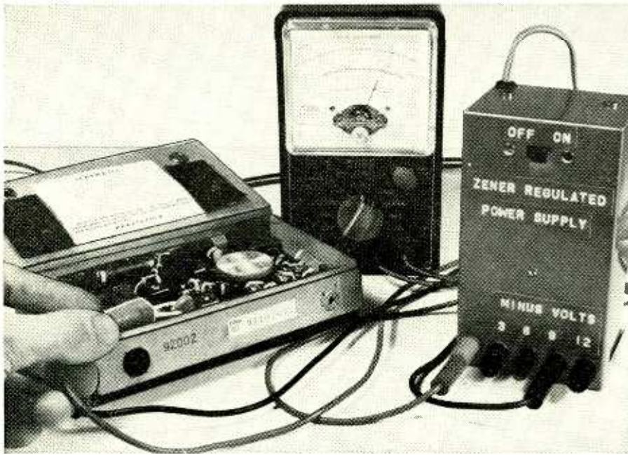
Supply being used to replace 9-volt round battery in transistor portable. Meter shows current drain to be about 7.5 mA.
