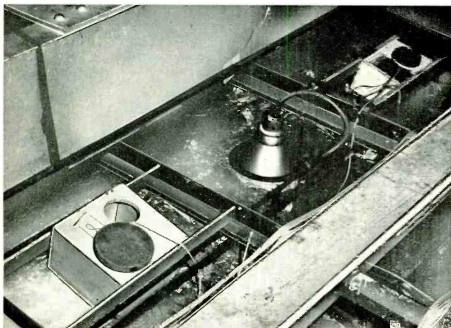
Two box type Helmholtz resonators (of lower Q than tubular type) fitted to speakers. "Funnel" between is lighting assembly.
