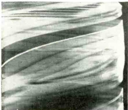
Fig. 10—Partially shorted yoke in direct-drive circuit.
