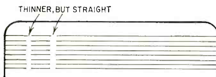
Fig. 6—False ringing. Trouble is on left side, but scanning lines are straight. Vertical lines are caused by scanning lines being thinner, or completely missing.
