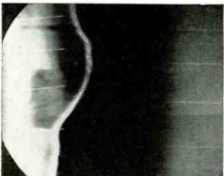
Fig. 11—Arc inside yoke. Radiation got into rf input.
