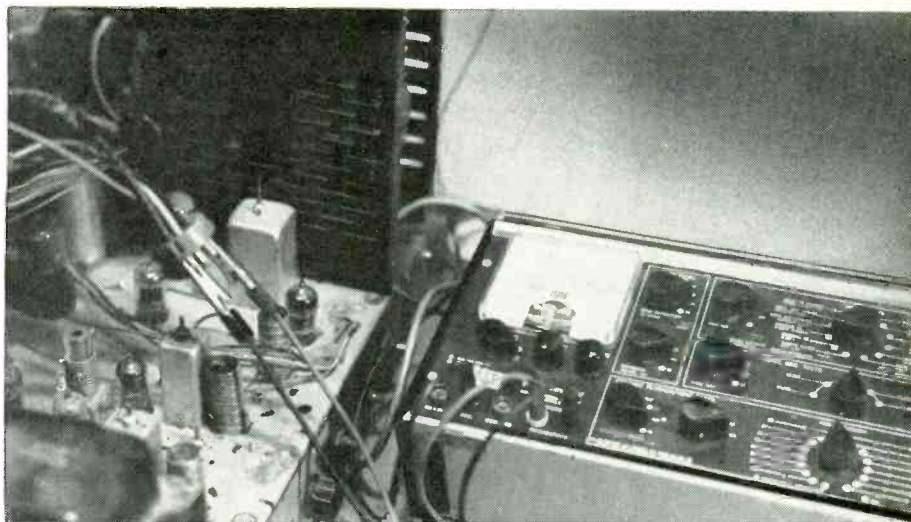
Fig. 9—Sweep-circuit tester with variable inductance used for checking yoke for trouble.
