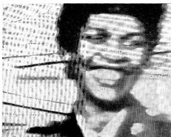
Fig. 1—The picture looks like this when the tube gets weak. But video trouble can also cause this kind of thing.
