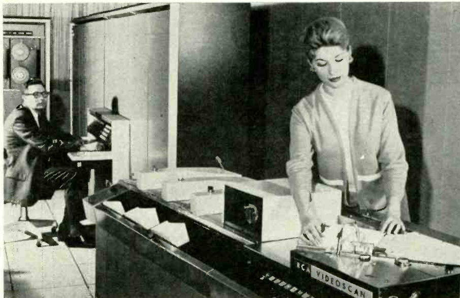
Gloria Duraczynski, of RCA, loads the input stacker of the Videoscan. Bills run along the track at the rear, past the TV tube in central housing. Part of the RCA 301 is in the background.
