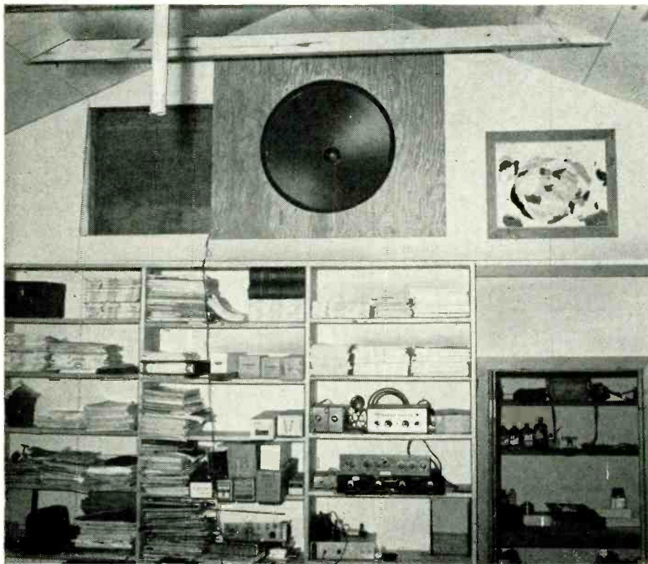
30 inches of woofer in wall of Marshall's laboratory. Back wave is absorbed in unused attic.
