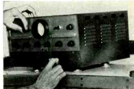
Electro-Nuclear D-X Navigator gives Loran system delay time in \mu sec.
