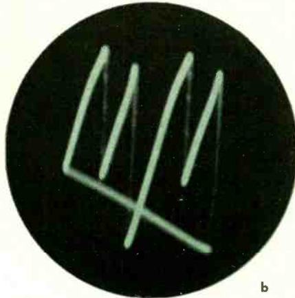
Fig. 3-a—Cyclogram with two basic excursions. b—Input waveform associated with cyclogram.
