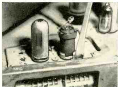
Seven-pin socket adapter plugged into TV tuner. Note single capacitor connected from grid to plate pins.
