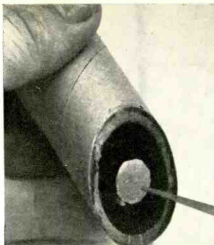
Aluminum-foil diaphragm is cemented to center of Saran wrap.
