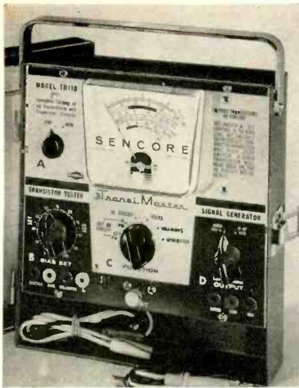
The Sencore model TR110 in-circuit transistor checker.
