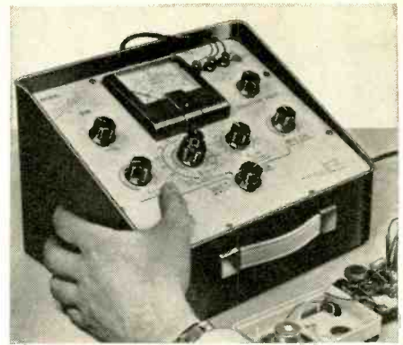
The Hickok model 890 in-circuit transistor checker.
