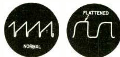
Fig. 7—Bad grid-drive waveform kills high-voltage.
