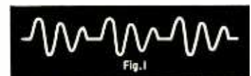
Fig. 1 illustrates crudely the type of vibration that results. Each shock pulse starts a new train of decaying waves.
