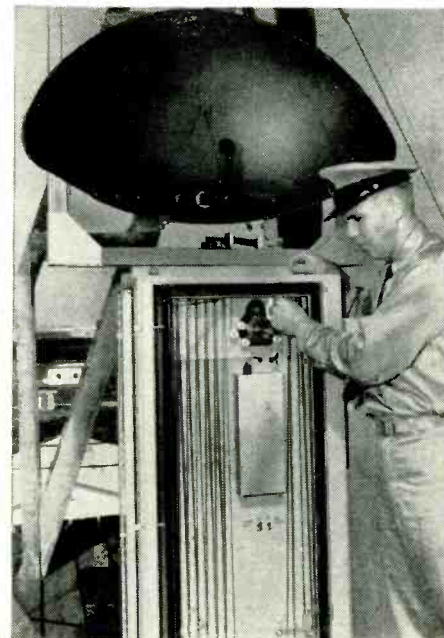
Coast Guard electronic technician chief Donald Actis adjusts the talking beacon transmitter on the New Jersey coast. Strips of talking tape and playback head are seen in the cabinet.
