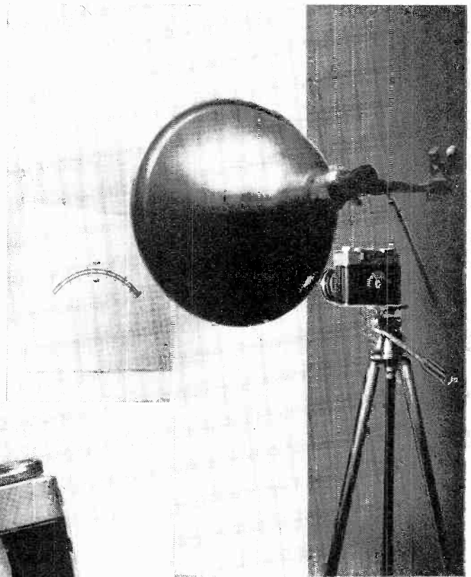
Fig. 3—Pin or tape the drawing to a suitable background such as a sheet or a white wall. (Second light is out of sight at right.)
