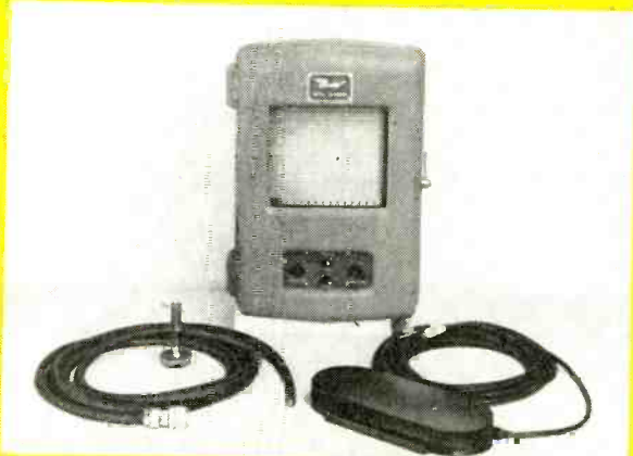
Bendix recorder. Right: double type transducer. Left: power cable, "stuffing tube" seals transducer cable passing through hull.
