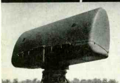
Vigilant acquisition radar for Nike-Hercules first detects approach of distant aircraft, pinpoints its location and instantly signals to battery control.
