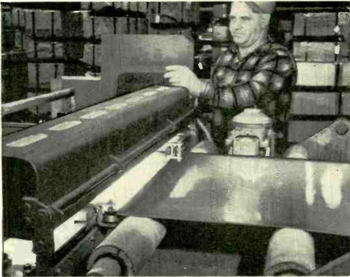
Electronic hole detectors on the Weirton tin mill cutting line detect holes as small as 1 millimeter in diameter (which can't be seen by the eye) and automatically reject defective sheets. The process is controlled by photoelectric cells.
