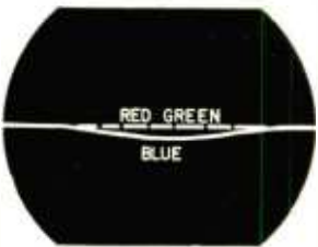
Fig. 7—Fundamental sine wave is adjusted in phase to peak blue line at center screen.
