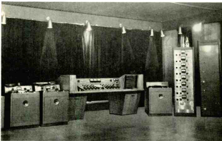
A small portion of the studio. At left are two standard Ampex tape recorders; center is the Monster; at its right the Octopus, flanked by its eight amplifiers and—at the extreme right—the power supplies for the equipment.
