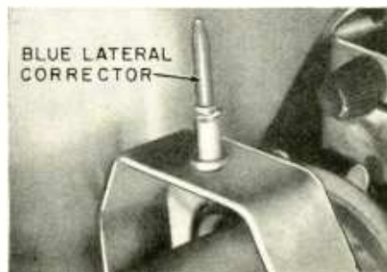
Fig. 1—A typical beam magnet is a PM unit with a control knob. It is rotated to obtain center-screen convergence. Note the dynamic convergence coils below the magnet.
