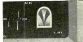
Precision-ray tuning eye makes it simple to tune precisely on both AM and FM.
