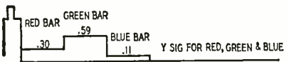
Fig. 13—Compatibility of color-TV and black-and-white TV requires that the Y signal as used in black-and-white transmission be unaltered.
