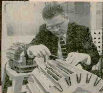
Dick trouble shooting Magnetic Drum Frame.
