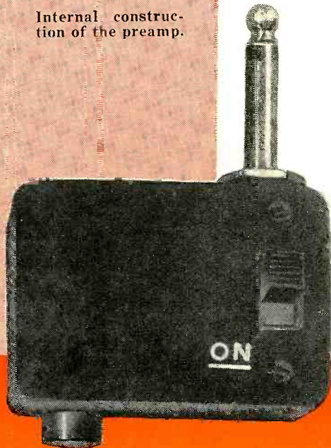
Phone plug adapts the preamp for use with most kit type meters.
