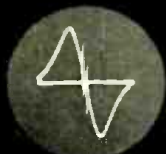
Narrow-band marker for S-curve observation
