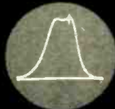
Wide-band marker for tuner alignment
