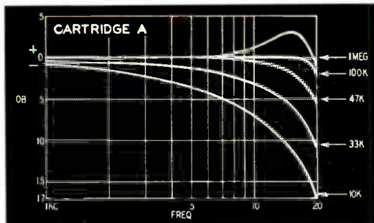
Fig. 1—Frequency response vs load of moving-coil cartridge.
