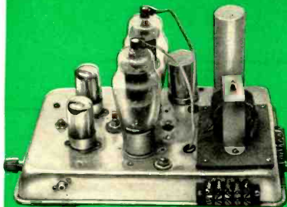
← The amplifier using a universal replacement type of output transformer.
