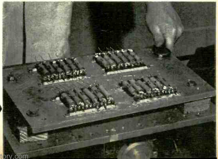
Oil-filled capacitors are subject to vacuum under elevated temperatures, then are individually examined to insure complete hermetic seal.
