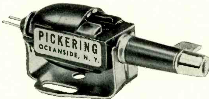
The Pickering Flux-valve pickup, with the plastic inserts removed.
