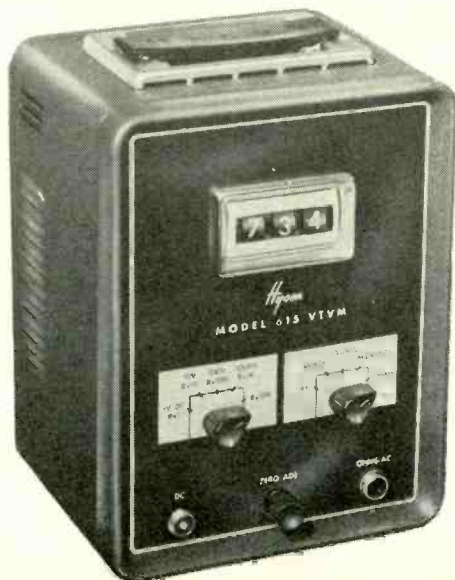
The Hycon model 615 digital vtvm with a close-up of the drum-type dial mechanism.
