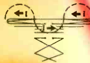
Current Distribution (Channels 7-13) Without Helix
