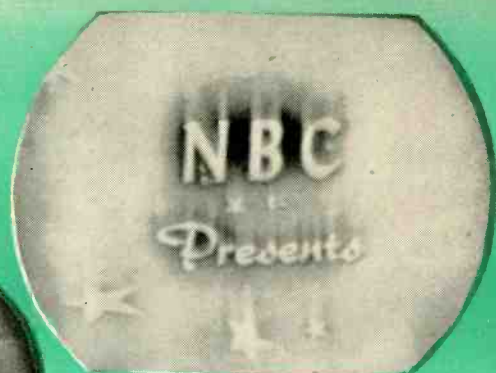
Fig. 2—Vertical picture bounce.
