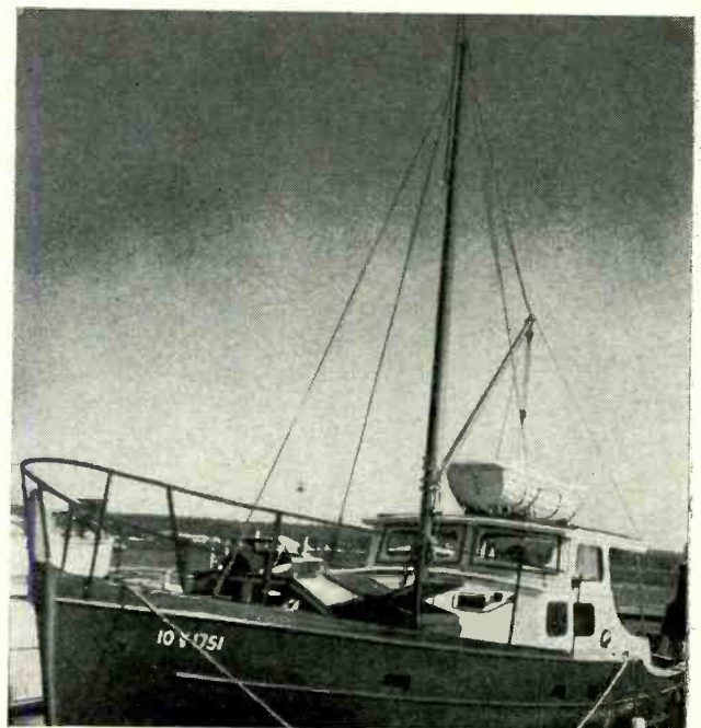
An ideal case. Antenna is strung from top of mast.
