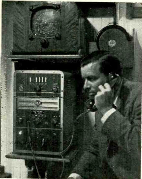
30-watt 6-channel radiotelephone and all-wave receiver in schooner cabin.
