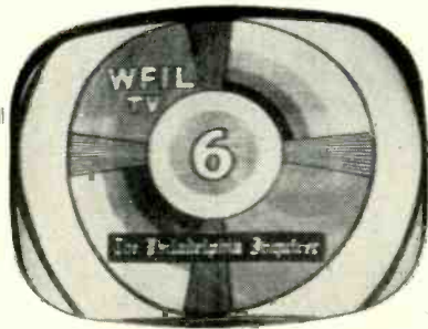
Fig. 4—High frequency sideband loss.
