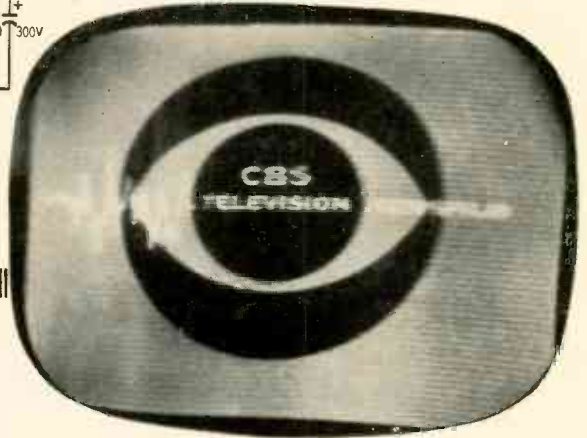
Fig. 2—Insufficient low-voltage supply.
