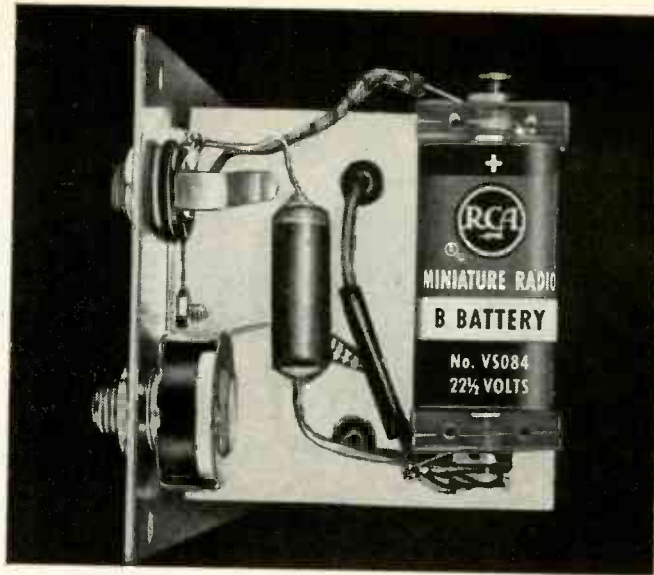
Under side of the novel code oscillator.
