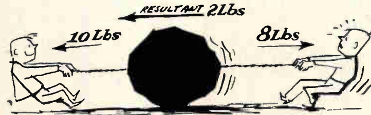
Fig. 2—Two forces acting on one object. The net acting force is the difference.
