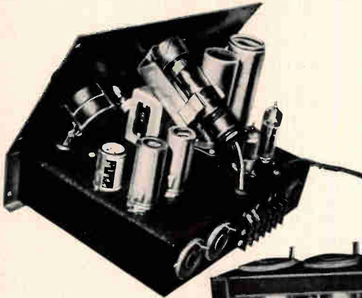
Left. Top view of remote amplifier. Ample room provides for neat layout.
