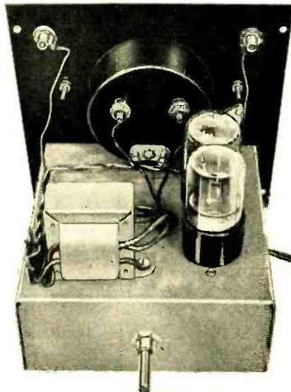
Fig. 3—Inside top-chassis view of the standard-model psychometer. The control at the back of the chassis is the static-balance potentiometer ( R_{12} in Fig. 2, reset at start of therapy.
