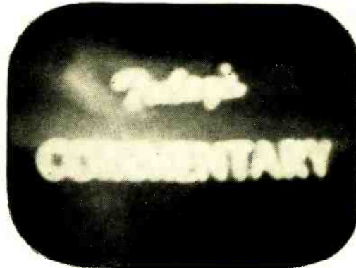
The result of intermittent defocusing in a Fada projection-type TV receiver.
