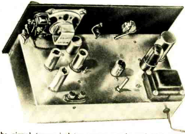
Layout of the signal tracer isolates power supply and high-gain amplifier.
