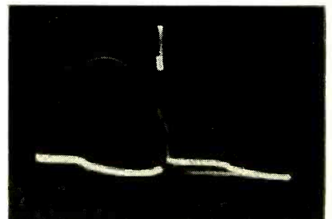
Fig. 11—Normal 6-kv flyback pulse at plate of horizontal-output amplifier. The capacitance-divider probe attenuates the pulse by a factor of 100 to 1 to avoid damaging the scope input circuit.
