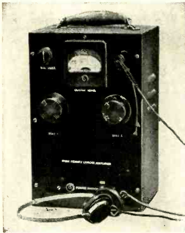
Fig. 1—The portable two-channel remote broadcast or recording amplifier.
