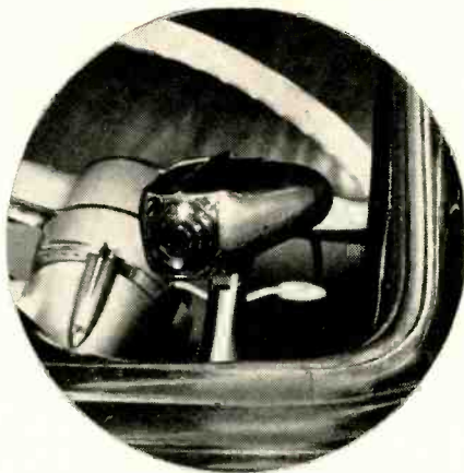
Photo A—The phototube unit mounts behind the windshield on the left side of the instrument panel. The prismatic lens concentrates light on the phototube.
