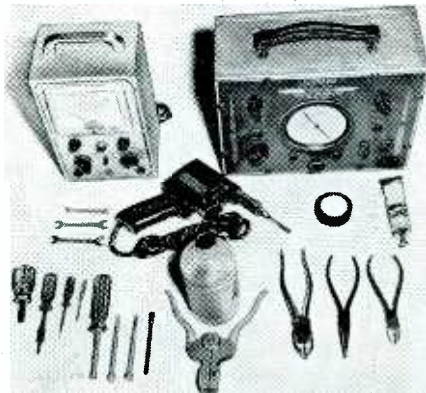
A v.t.v.m. (or v.o.m.), signal generator, soldering iron, and an assortment of hand tools forms the basic equipment needed to begin a radio repair business.
