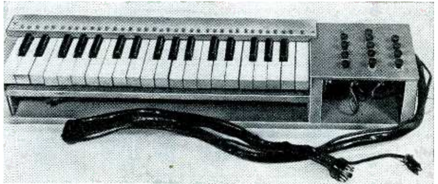
↑ Photo A—Thirty-seven keys control the 5-octave range of the Thyratone. Buttons at right are used to select the tone color combinations.
