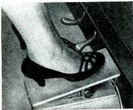
Photo C—Volume of the music is controlled by this specially made expression pedal. It rests on the floor in a convenient position for the player's foot.
