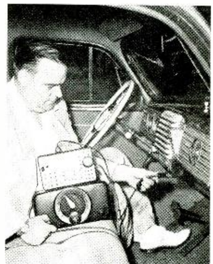
The author plugs a converter into a car lighter. The receiver is a Zenith Major.
