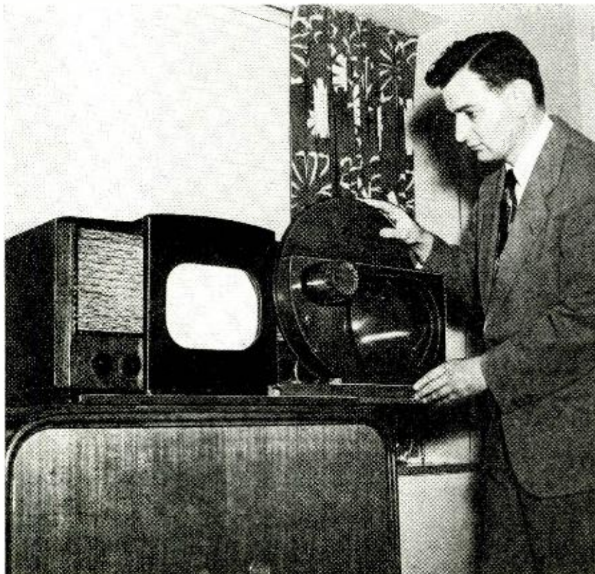
A spinning color wheel must be put in front of the screen in the CBS system.
