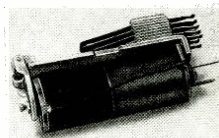
Fig. 4—A slow-release relay. The copper slug covers the coil's heel end.
