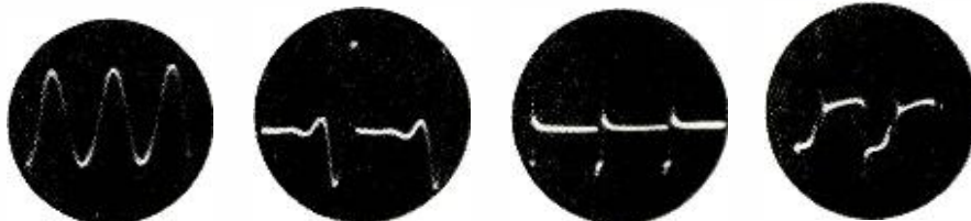
These oscillograms show what happens when feedback in a conventional oscillator is too great and when the time constant of the grid-leak is too long. The perfect sine wave results when feedback is reduced to the optimum value by any of the methods illustrated in Figs. 1-c through 1-f, or by using a suitable transformer.
