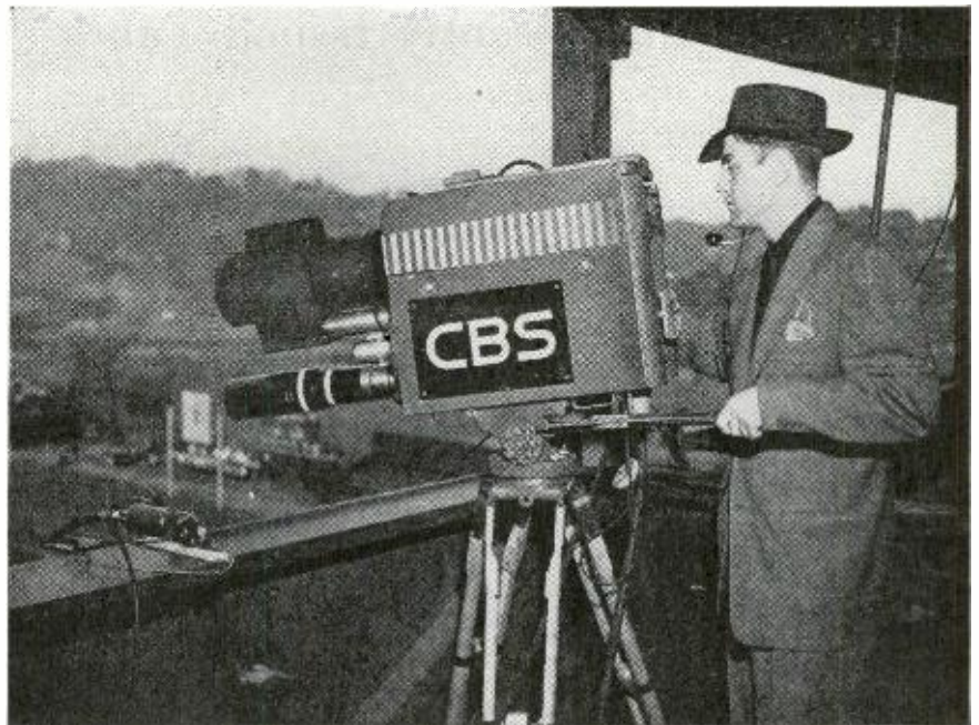
The 40-inch focal length lens is no longer than other standard TV camera lenses.
