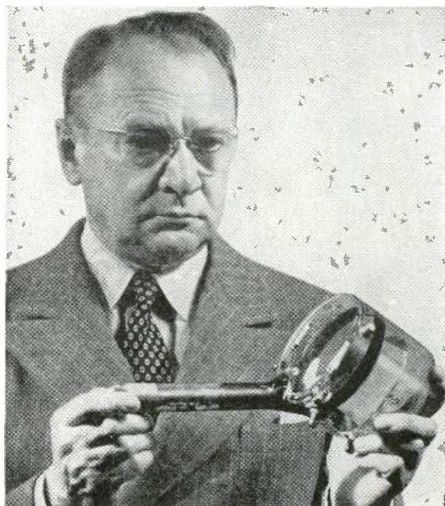
Dr. V. K. Zworykin of RCA Laboratories with his iconoscope tube. Its successor, the image orthicon, has been developed by RCA scientists to have up to 1000 times greater sensitivity.
